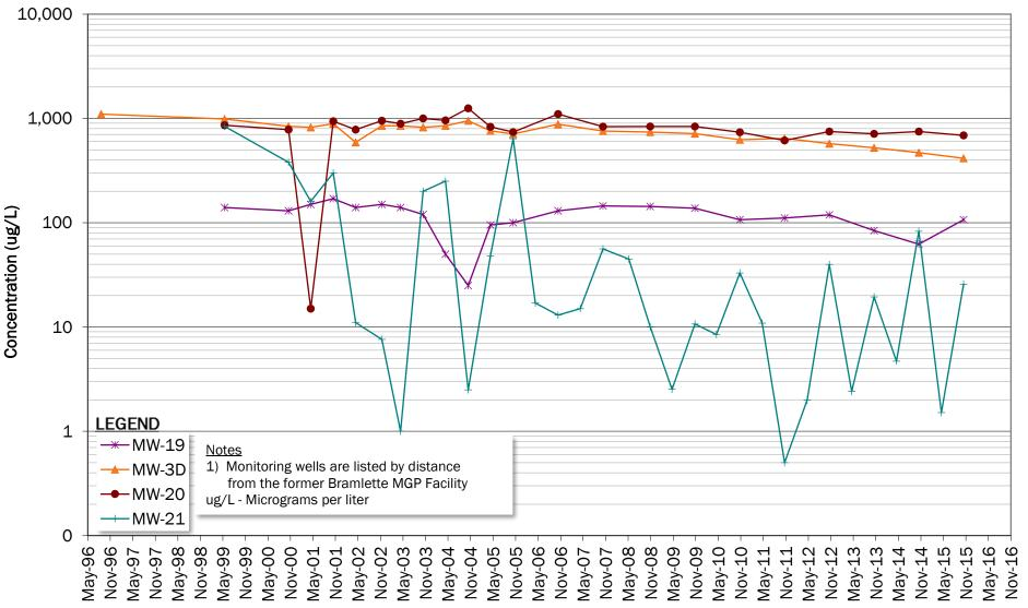
Figure 6C Former Bramlette MGP Facility Naphthalene Concentration Trend Plot Shallow Wells
