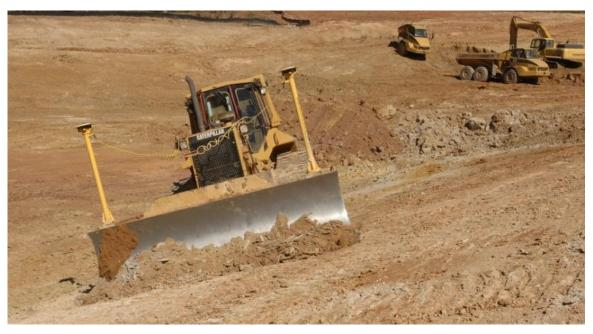
Figure A-16 Dozer with GPS Controls (Foreground), Articulated Trucks and Excavator (Background)
