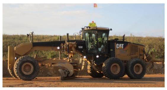
Figure A-14 Motor Grader Source: Haile 2018.
