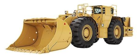
Figure A-34 Typical Load-Haul-Dump Unit (LHD) Source: Caterpillar
