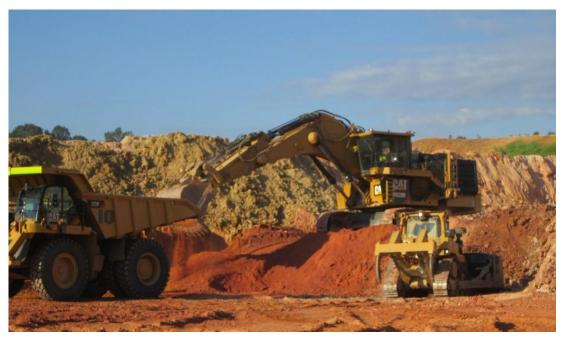
Figure A-12 Hydraulic Excavator, Dozer, and Haul Truck Source: Haile 2018.
