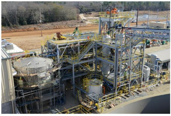
**Figure A-54** Elution Circuit – Acid Wash, Barren Tank, and Carbon Regeneration Rotary Kiln Source: Haile 2018.
