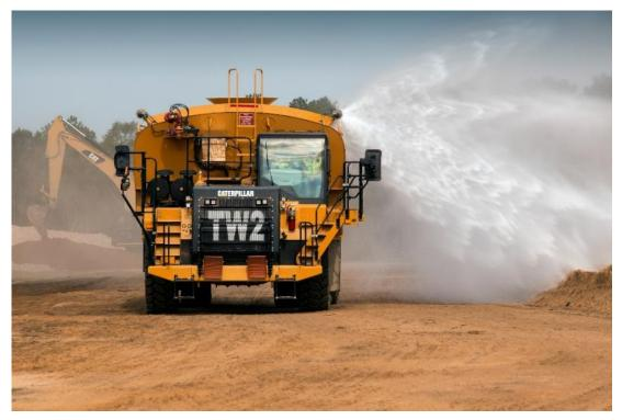
Figure A-15 Water Truck for Dust Control Source: Haile 2018.
