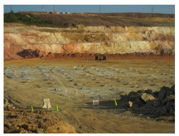
Figure A-11Drill Holes in a Blast PatternSource: Haile 2018.
