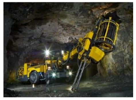
Figure A-35 Typical Down-the-Hole (DTH) Drilling Unit Source: Atlas Copco
