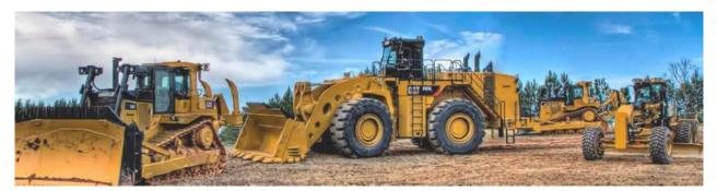
Figure A-13 Example of a Track Dozer (left and in background), Wheel Loader (center), and Motor Grader (far right)
