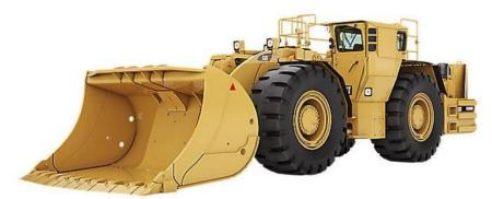
Figure A-34 Typical Load-Haul-Dump (LHD) Unit Source: Caterpillar
