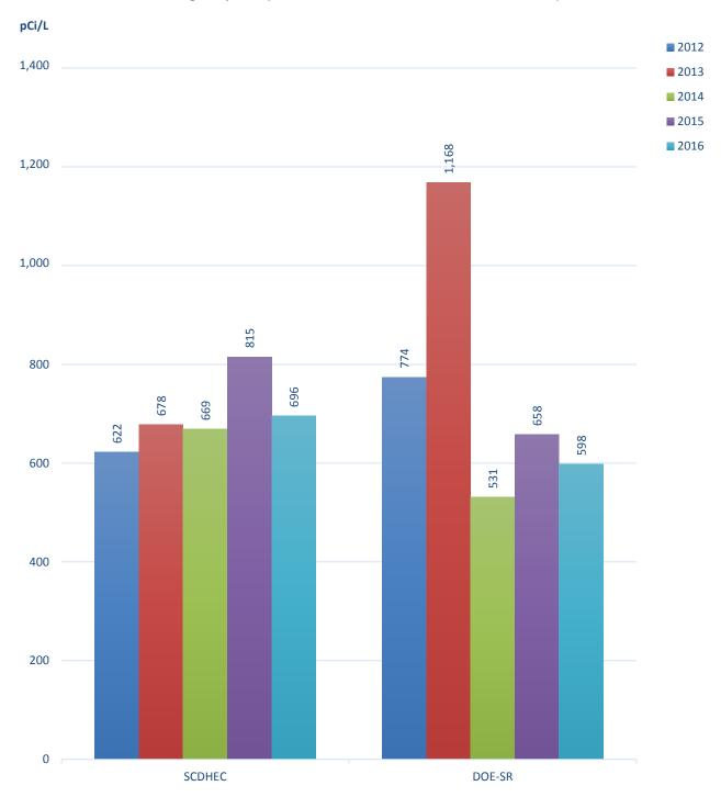
Figure 3. 2012-2016 Average Tritium Data Trends for DHEC and DOE-SR for Fourmile Branch at USFS Road 12. (SRNS 2013-2017, DHEC 2014a, 2015-2017)
