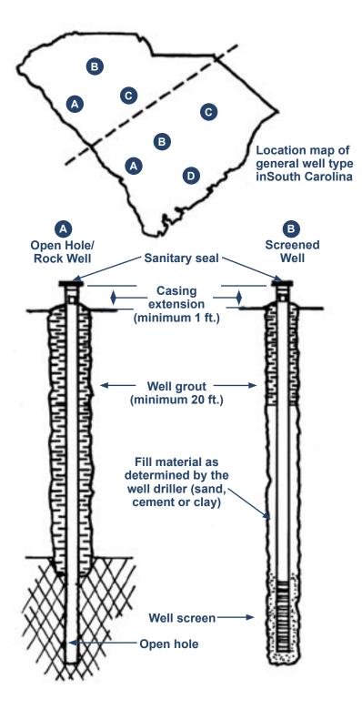
There are four types of wells typically found in South Carolina. In the northwestern portion of South Carolina, (A) open hole/rock wells, (B) screened wells, and (C) dug wells predominate. In the southeastern portion of the state, (A) open hole/rock wells, (B) screen wells, (C) dug wells and (D) jetted/driven wells can be found. The general construction details are shown in the accompanying illustrations.
