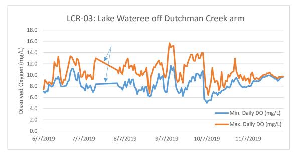
*Figure 3. Daily minimum (blue) and maximum (orange) DO concentrations (mg/L) observed at station LCR-03. Data between 7/17 and 7/31 (arrows) are not included due to a combination of an improperly functioning sensor and data loss of a partial record.*
