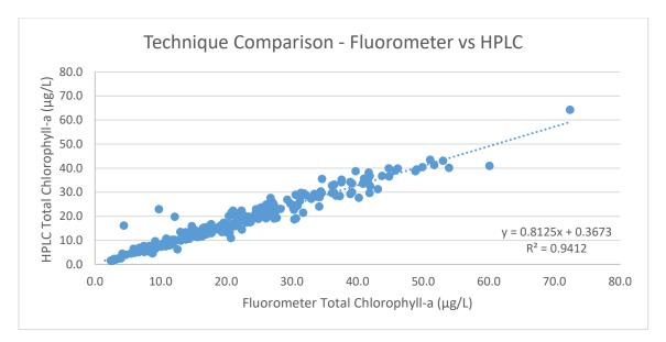
Figure 9. Comparison of total chlorophyll-a concentrations determined using fluorometer and HPLC techniques.
