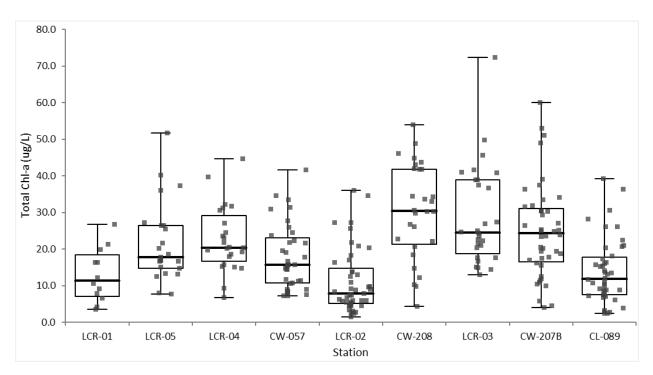
Figure 10. Box plot summary of all fluorometric total chlorophyll-a measurements for each station. Data were collected between late April and late October on a biweekly sampling schedule.
