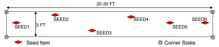
Figure 6 Test Strip Conceptual Layout
