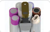
Wiper keeps sensors clear of biofouling
