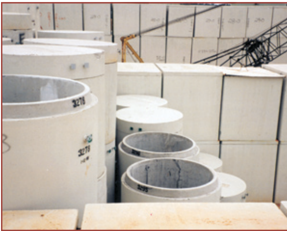
A typical configuration of cylindrical and rectangular A Trench disposal vaults. The vaults are configured to ensure trench cap structural integrity and to reduce radiation exposure to workers during LLRW off-loading activities.
